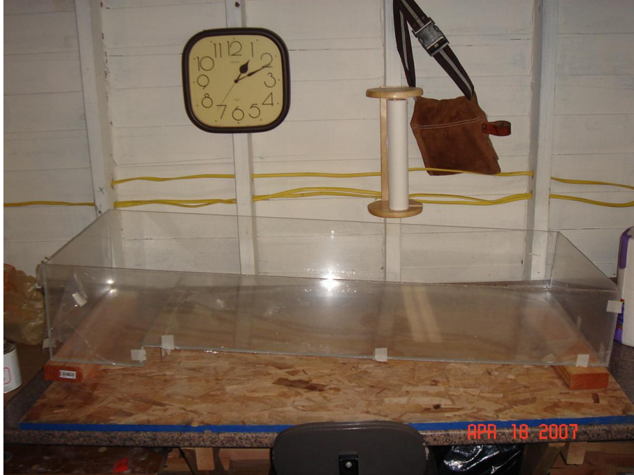
Figure 3: Finished Lexan® enclosure for the dam model. *Note* – Lexan® brand clear silicon sealant was used on the inside of enclosure at each joint after solvent had completely dried to ensure a water-tight seal.
