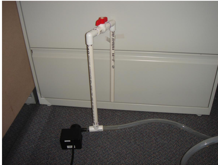
Figure 21: Pump setup that is placed in a bucket directly beneath the outlet from the model. *Note* The chosen pump had only limited ability for flow adjustment. It was found that the flow could not be regulated adequately for the purposes of this project, therefore a by-pass utilizing ½ inch (ID) PVC piping and PVC ball valve was added to allow for full regulation of flow. (This also allows the demonstrator to adjust flow without reaching entire arm into the bottom of the bucket!) The pump used for this model is a landscaping pond pump (Beckett Corp. M400AUL).
