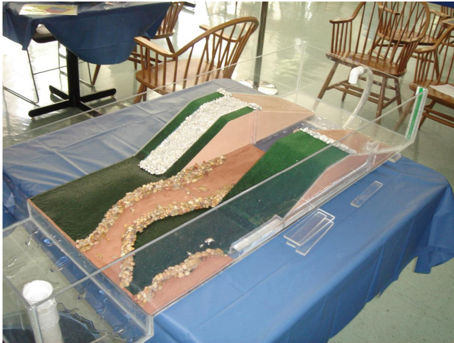
Figure 24: Model ready for demonstration. Note the small pieces of Lexan® next to the model are used as flashboards and also to force flow over the emergency spillway or to increase head on the primary spillway drop box.
