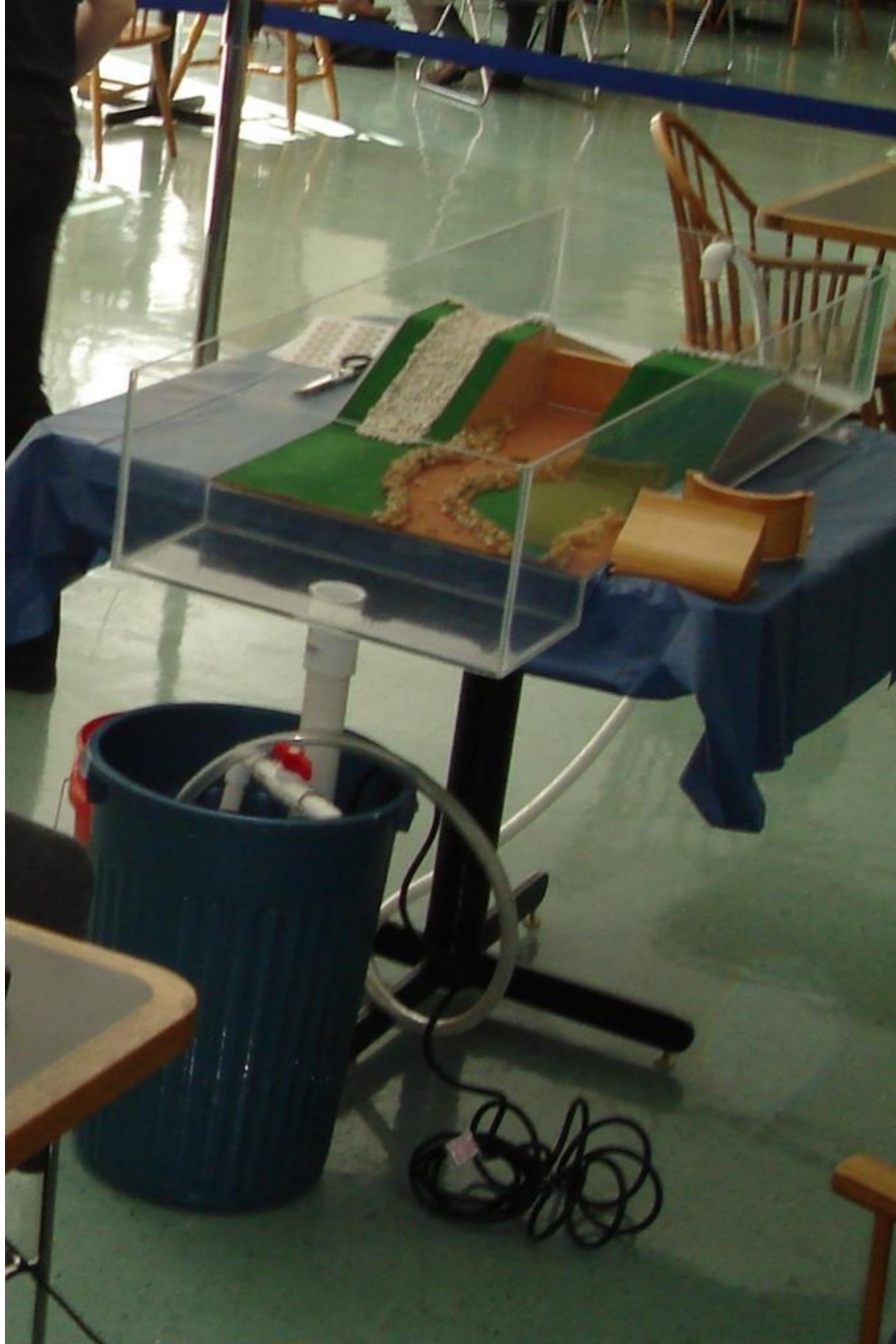
Figure 23: Fully assembled model ready for demonstration. Obvious caution should be taken when using the model and water around electricity. GFCI protected wall outlets/extension cords should be used for the pump for safety purposes (no floor outlets in case of spill).
