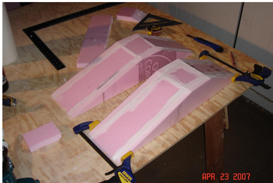
Figure 4: Dam embankment made from a sheet of rigid foam insulation and assembled with caulk. *Note* – dam can be constructed from whatever material is deemed appropriate (i.e. solid foam block, modeling clay, etc.). This assembly procedure was a bit tedious and time-consuming!
