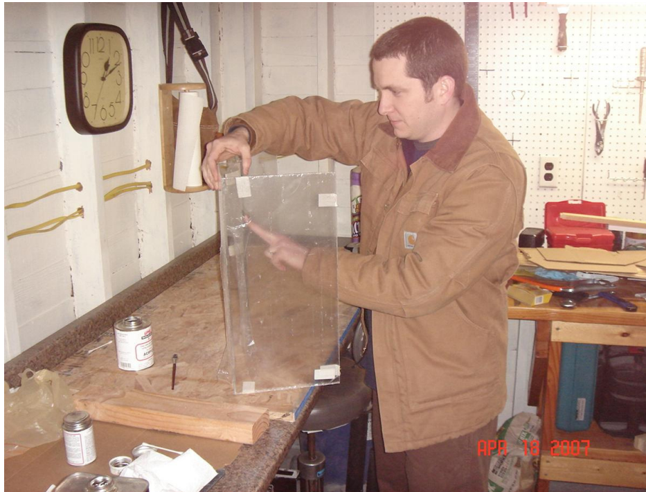
Figure 1: Assembling Lexan® enclosure by joining pieces with solvent cement.
