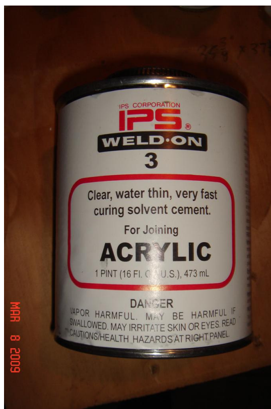
Figure 8: Solvent cement used for assembling the Lexan® enclosure.
