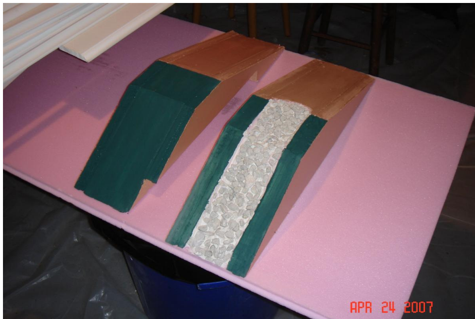
Figure 6: Painted embankment sections (later 'grass' was substituted with self adhesive matting material for aesthetic purposes). Note the cutout section in the left embankment section above for installation of the primary spillway drop box structure and discharge pipe (see Figure 7, and 11).
