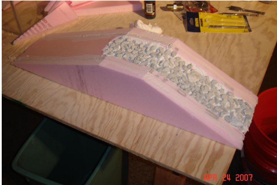
Figure 5: Construction of emergency spillway channel with clean stone and caulk serving as 'grouted riprap'. *Note* Silicone caulking should be used as opposed to latex.
