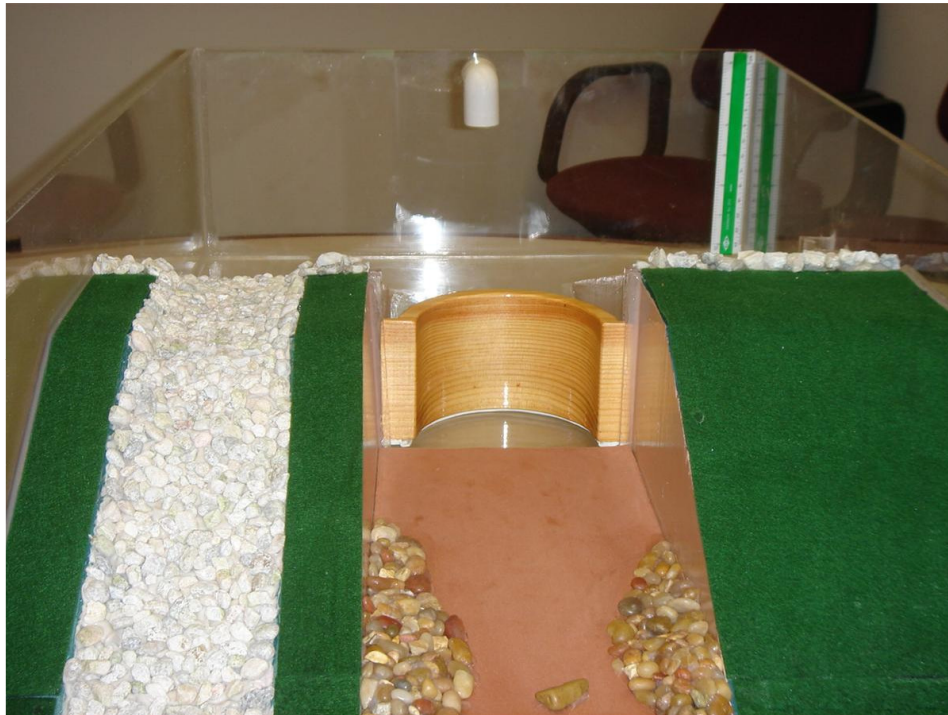
Figure 13: Semi-circular spillway weir. *Note* The bottom of each spillway was lined with pieces of self adhesive weather stripping to ensure a seal between bottom of spillway and enclosure.
