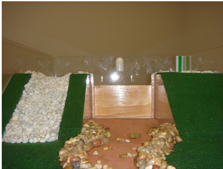
Figure 12: Longitudinal view from outlet channel looking ‘upstream’ showing elevation differences between dam crest, emergency spillway and secondary spillway weir (the primary spillway in this model is the dropbox structure shown in Figures 7 & 11, but cannot be seen in this photo).
