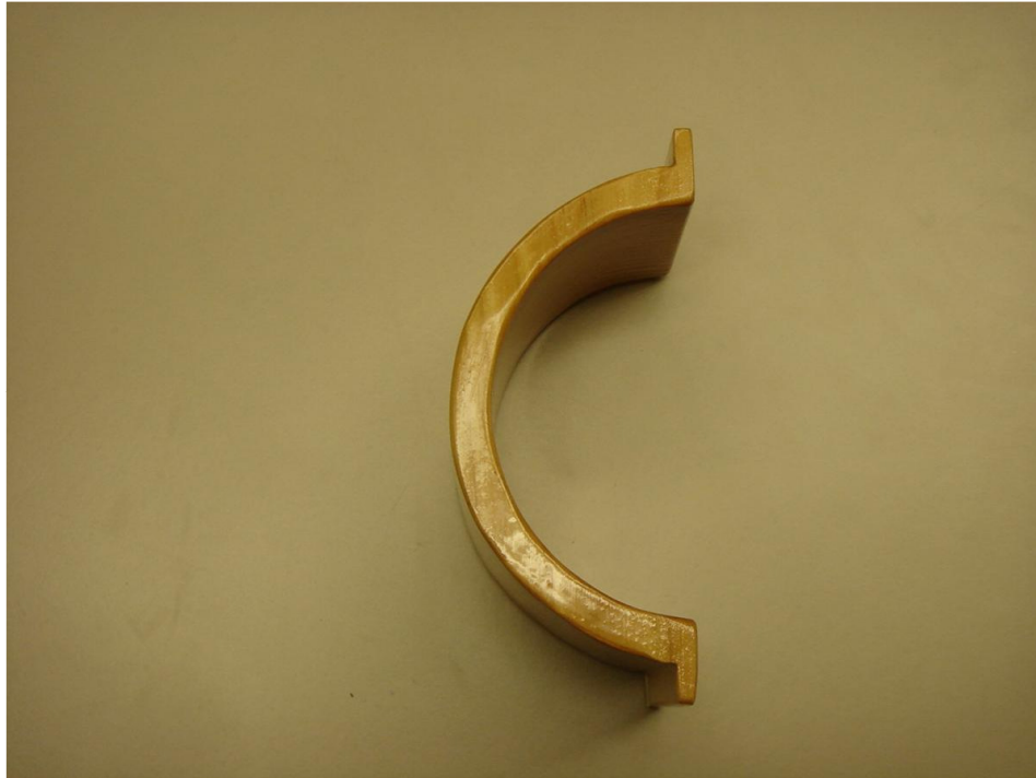
Figure 14: Plan view of semi-circular spillway weir. *Note* Tabs at each end were designed to fit into the guides described in Figure 12.
