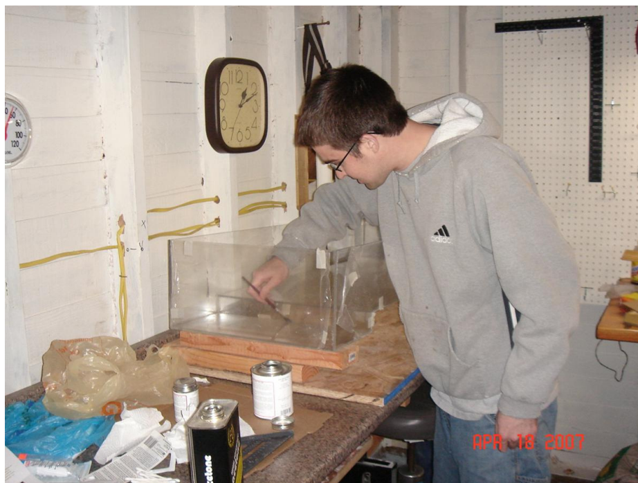
Figure 2: Applying additional solvent cement to all joints to ensure adequate adhesion.
