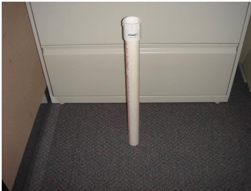
Figure 22: Discharge pipe with 1 ½ inch PVC female threaded fitting to be attached to the fitting shown in Figure 20 and placed into the bucket beneath the model (to make sure all water makes it back into the bucket).
